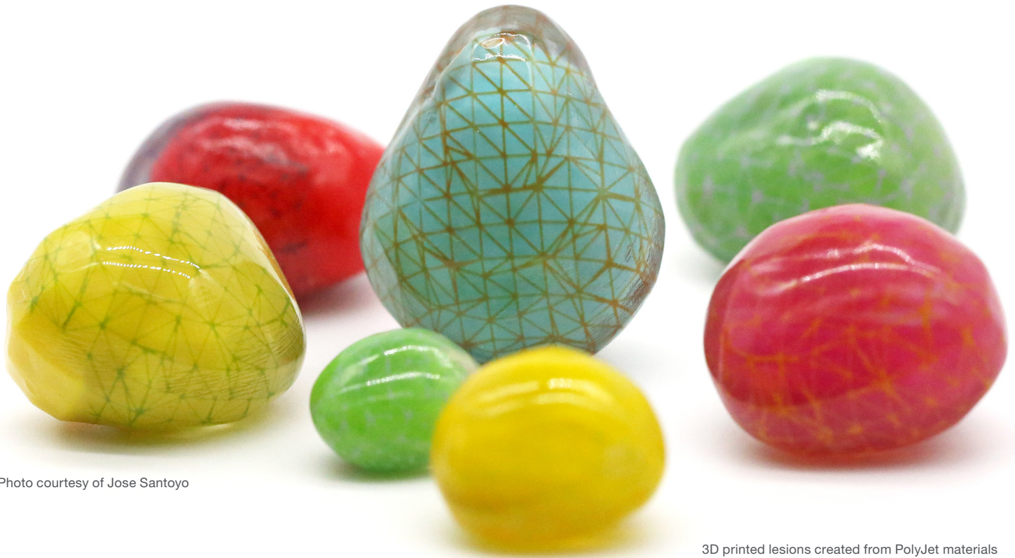
3D printed lesions created from PolyJet materials that allow for the modeling of change over time
